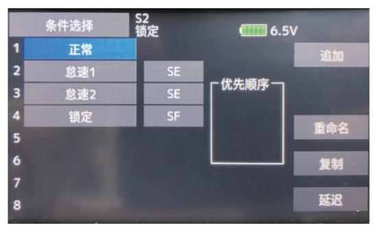
4. 设置 CH5 为起落架模式,设置开关用于控制姿态模式/3D 手动模式切换 Set CH5 as landing gear mode, and set the switch to control attitude mode/3D manual mode switching
